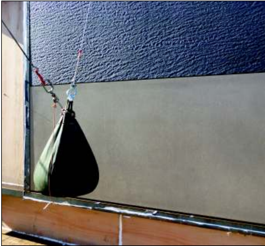
SOFT BODY IMPACTOR READY FOR RELEASE
