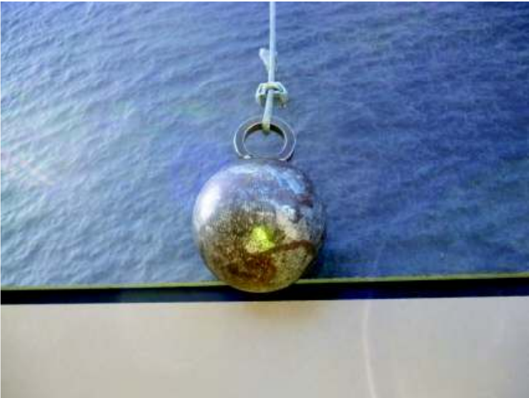
HARD BODY IMPACTOR ON UPPER PANEL
