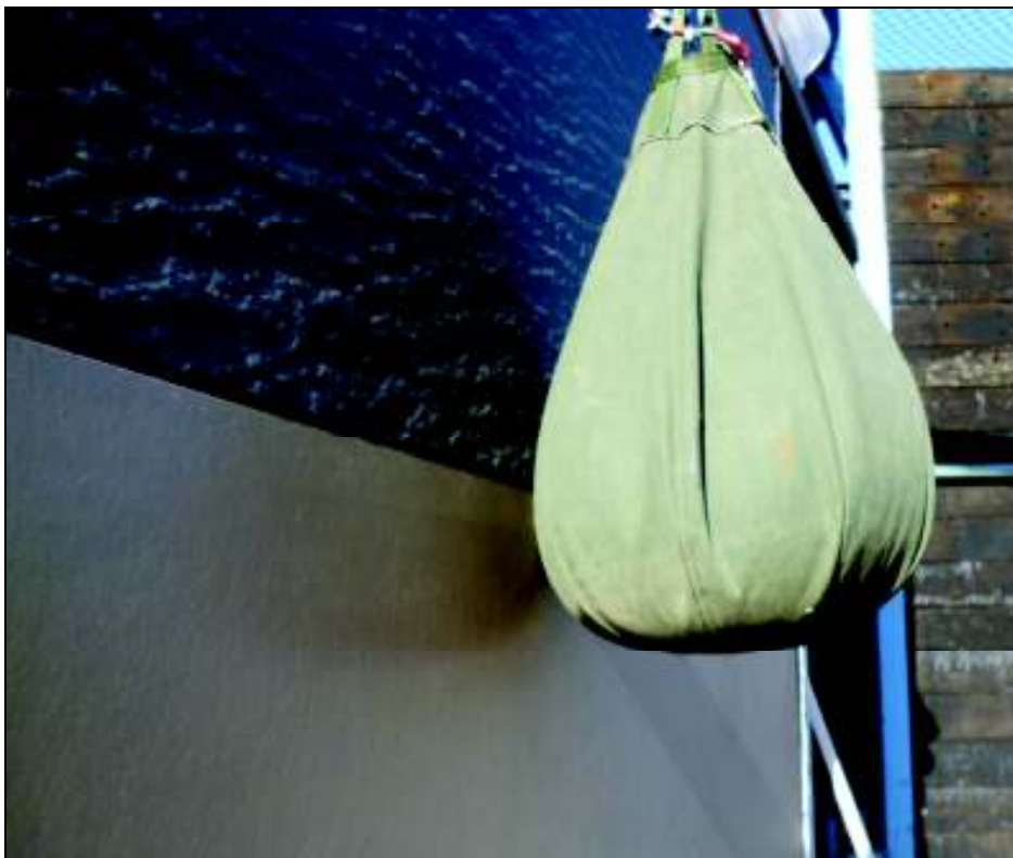
SOFT BODY IMPACTOR ON PANEL JOINT
