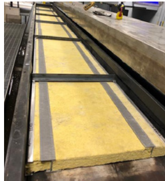
ASTM E84 is the standard test method for assessing the surface burning characteristics of building products to observe the flame spread and developed smoke density. The above photos show the STRONGIRT® and mineral wool insulation assembly before and after testing.
