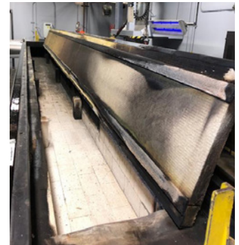
ASTM E84 is the standard test method for assessing the surface burning characteristics of building products to observe the flame spread and developed smoke density. The above photos show the STRONGIRT® and mineral wool insulation assembly before and after testing.
